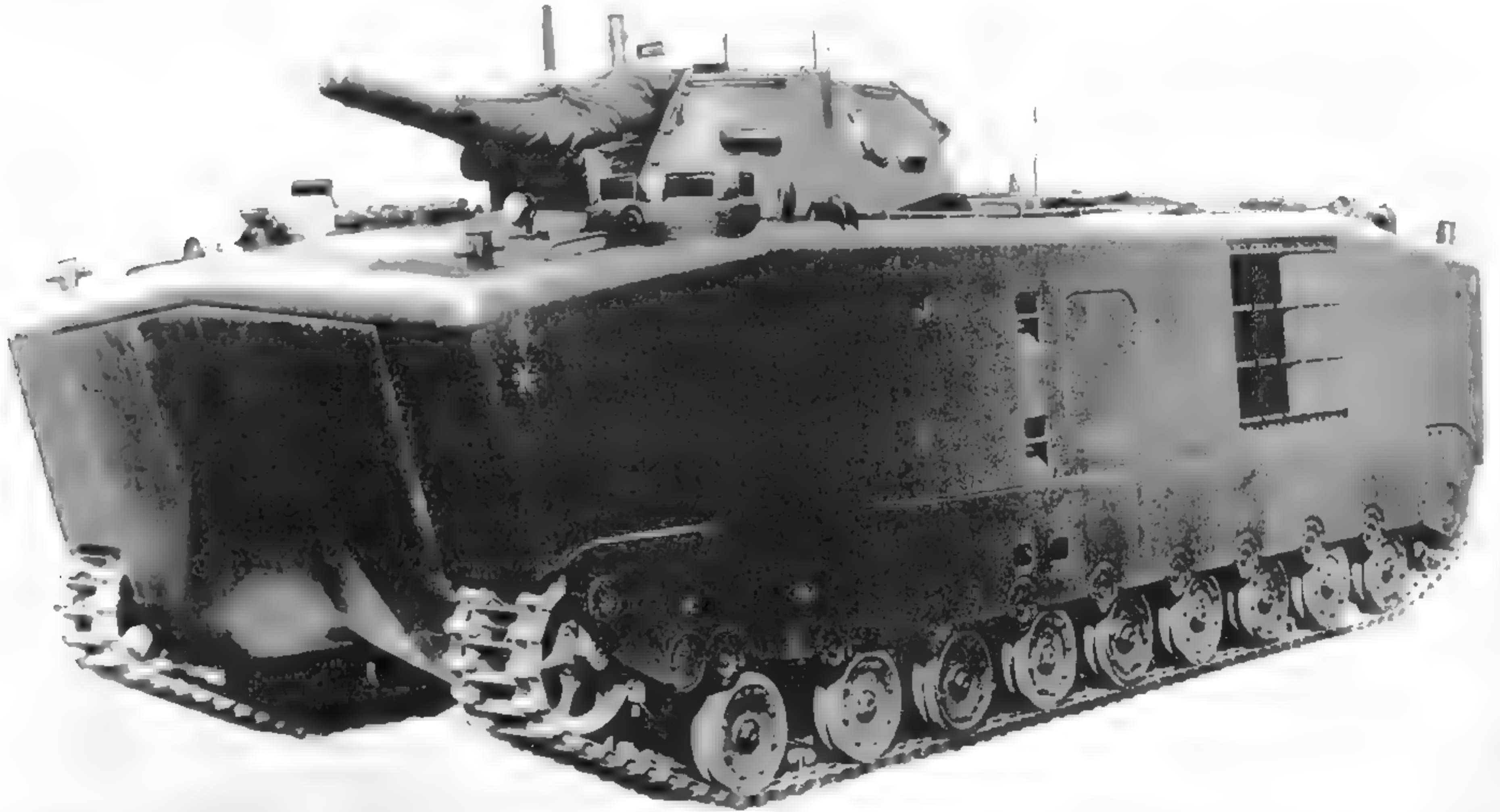
The LVTH6 provided amphibious troops with needed artillery support. A .30-caliber machine gun was mounted coaxially with the 105mm howitzer in the turret. (Photo courtesy of the Patton Museum)
